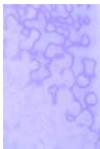
NEODYMIUM-RG B Pale Blue (changes to Pink under incandescent or natural lights)
